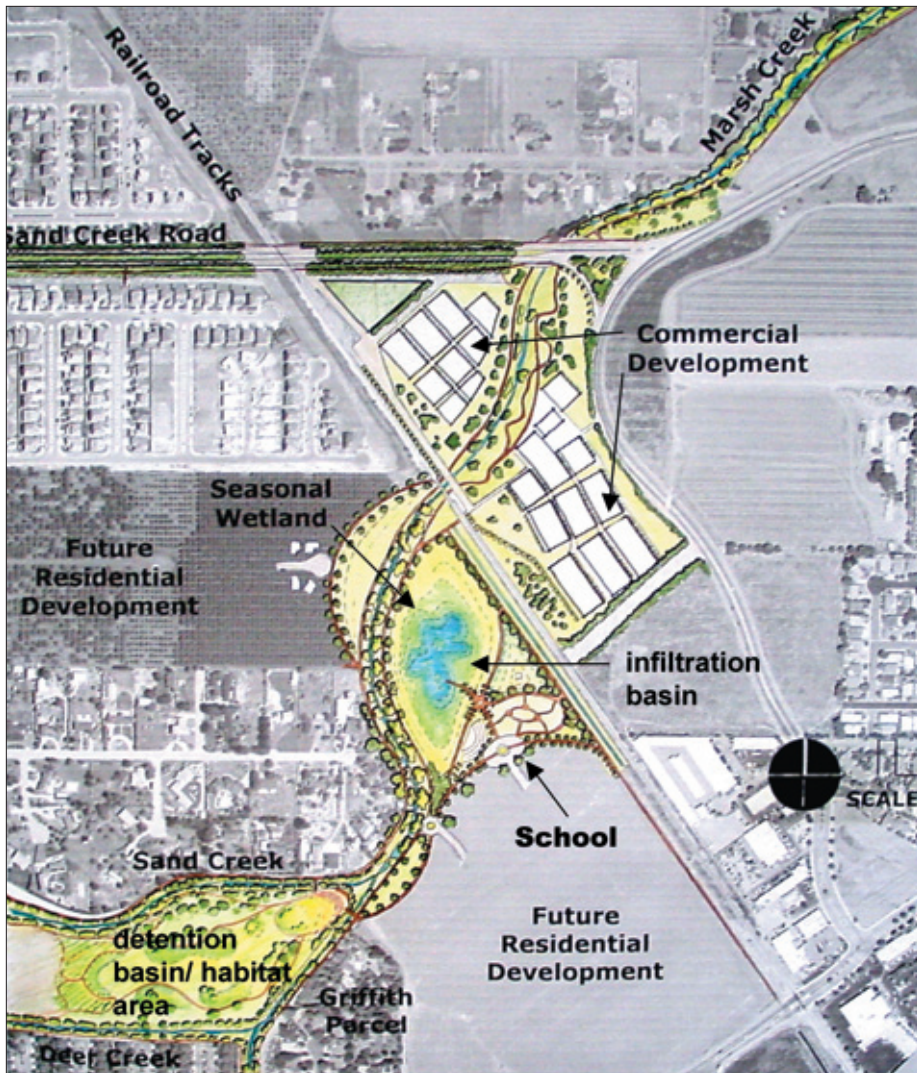
Figure 41 – Design to Reduce Polluted Runoff from New Development Design by UC Berkeley LAEP students.
