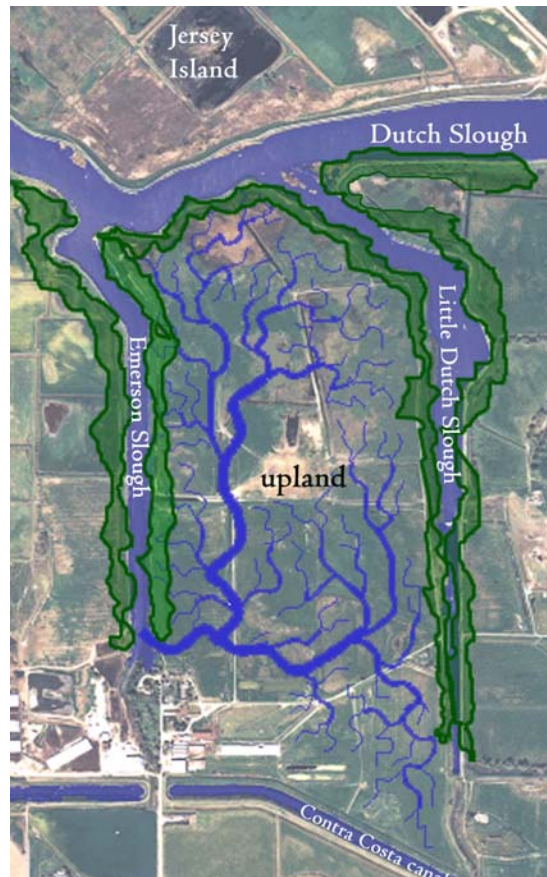
Figure 8: Representative design for the Gilbert parcel with dendritic channels in interior and riparian vegetation on the levees.
